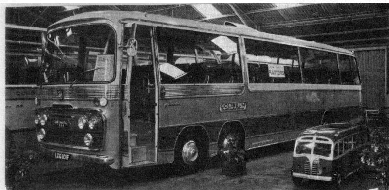
This is the Bedford VAL 70 Plaxton Panorama 1, specially designed for Continental touring. Unlike most Panoramas, it seats only 44, in reclining seats. The coach is equipped with the Telma electric retarder, and a two-speed axle.
